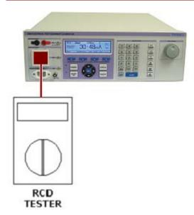
Residual circuit breaker testers manufactured by many companies are designed to test and measure the break time of AC mains (RCB) trips at set test currents. To do this they allow a fault current to pass between live phase and earth. The 'fault' current is started by pressing a button on the tester, usually an LCD counter on the tester measures the time in milliseconds until the mains supply is disconnected.
