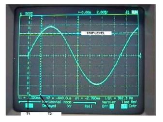
The diagram above shows the start of the fault current from an RCB tester. The test button would have been pressed at a point in the previous cycle PRECEDING the point T1 - up until then there would either have been no current or with some testers a PRE-TEST current below the trip current level.
